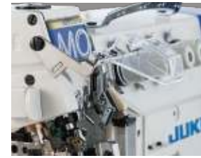
1. Eye guard with an open/close sensor
