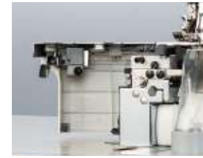
2. Cloth plate cover with an open/close microswitch
