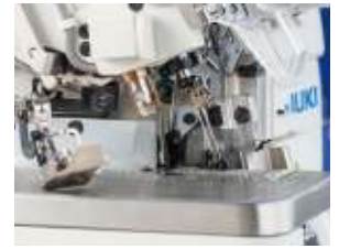
3. Presser foot arm with an open/close sensor
