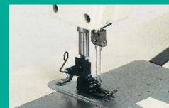
Tandem 2-needle double chainstitch machine WF=382
