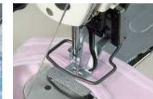
M type (Bartacking shoulder of running shirt)
