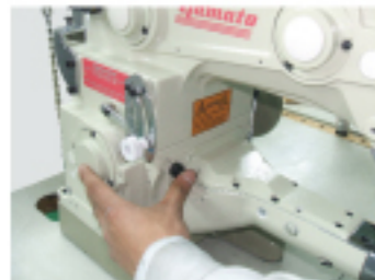
stitch length can be adjusted by pushing button easy & quick
