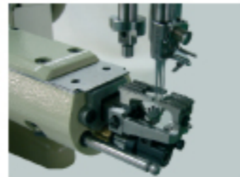
spreader locates on right side
