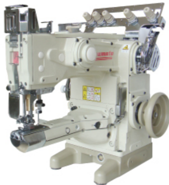
stitch length can be adjusted by pushing button easy & quick
