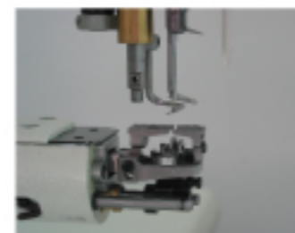
differential feed as standard "no wave" finish
