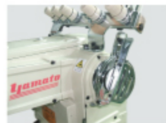
external thread take-up thread is supplied smoothly
