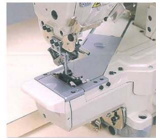
VG2708-WF8 1 needle cylinder bed double chain stitch machine for top stitching of display tape.
