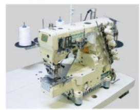
2, 3 Needle Cylinder Bet Interlock Stitch Machine for Hemming, with Left hand Fabric Trimmer Left hand Fabric Trimmer trims edge of fabric for neat finish.
