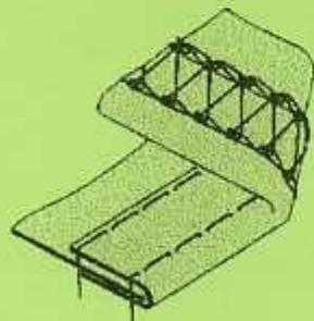
2 NEEDLE FLAT BED INTERLOCK STITCH MACHINE FOR LIP BINDING,
