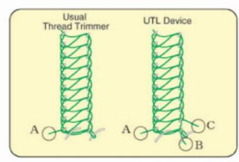
UTL device cuts the under thread at two points of "A" and "B" as the left picture. As "C" becomes the thread end, it prevents the seam from unraveling, unlike the case of only "A" is cut at the end of the
