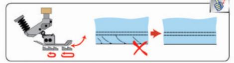
Walking Presserfoot can elimilate damage on fabric and present you "tunnel free" finish.
