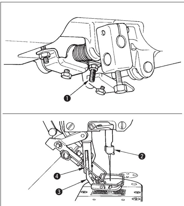
1) The standard height of the presser foot lifted using the knee lifter is 10 mm.
