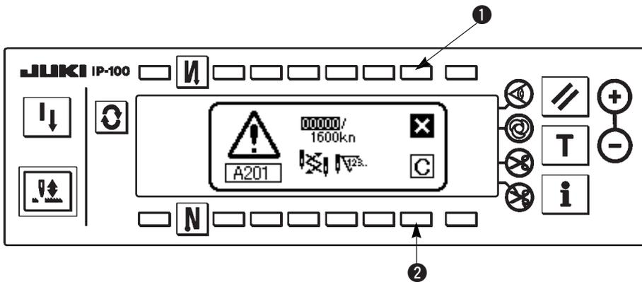
① : When ① is pressed, the screen can be cleared. However, the counter itself cannot be cleared. In case of the replacement of needle, the warning screen is displayed at intervals of 10 minutes until clearing is performed. In case of other warnings, the warning screen is displayed at the time of turning ON the power until the counter is cleared.
