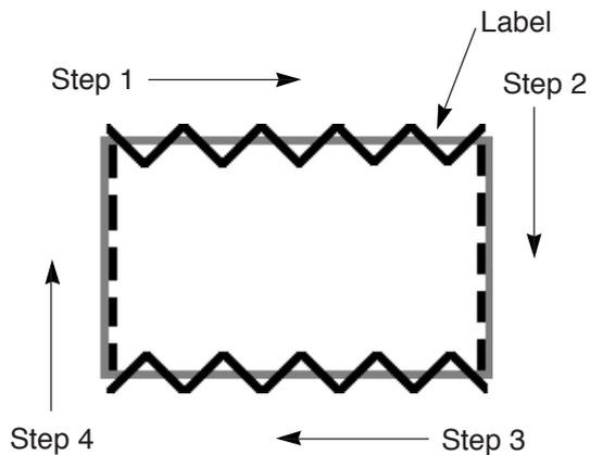
Example) In the process of label attaching, change over the zigzag patterns of constant-dimension stitching of standard zigzag stitch and straight stitch as shown in the figure, and perform the constant-dimension stitching.
