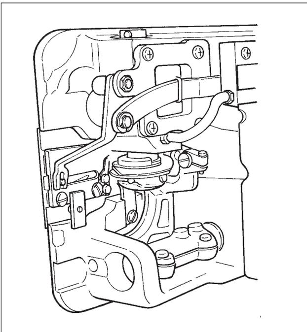
When cloth waste or the like gathers around or adheres to the hook section, trouble (defective sewing, seizure of hook, etc.) of sewing machine will be caused. Periodically clean the section.
