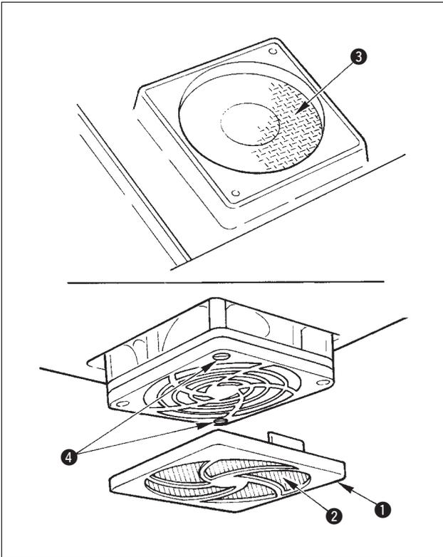
Cloth waste or the like gathers around the cooling fan filter section installed on the lower part of the under cover, and there is a case where cooling effect of the machine head is decreased.
