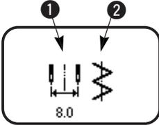
Max. zigzag width limitation value and reference of stitch base line are displayed when the power is turned ON.
