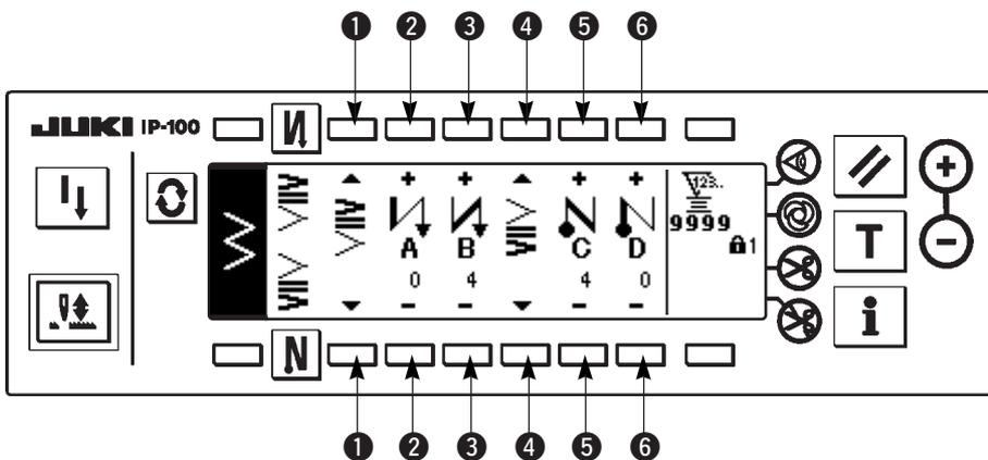
\* For the reverse feed stitching setting, there are two kinds of methods below according to the zigzag patterns.
