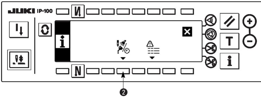
2) Press ② to display the maintenance function screen. (For other functions, refer to the Engineer's Manual.)
