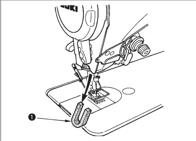
Remove needle bar stopper ① for transportation.
