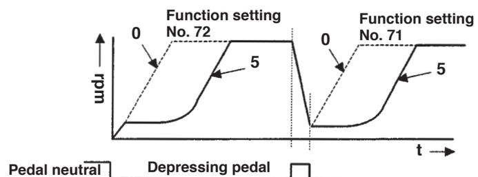
**18 Function of reducing speed of reverse feed stitching at the start of sewing (Function setting No.92 F-DSBT)**
