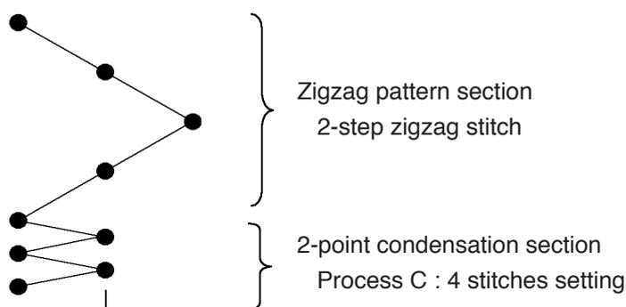
Compensation can be performed in the direction of “-”. (In case of the figure, the width narrows to the left side.)
