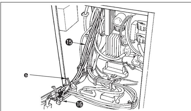
12) Insert white connector 6P three cords ⑮ coming from the machine head inside the electrical box through front cover through hole B, pass it through cord clamps "a" and "e", and insert it into connector CN54 ⑯.
