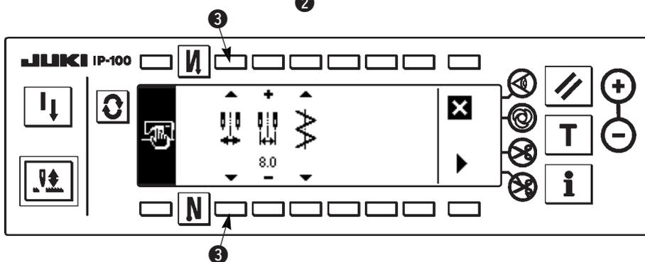
3) Figure on the left side is the zigzag width symmetrical in the center mode.
