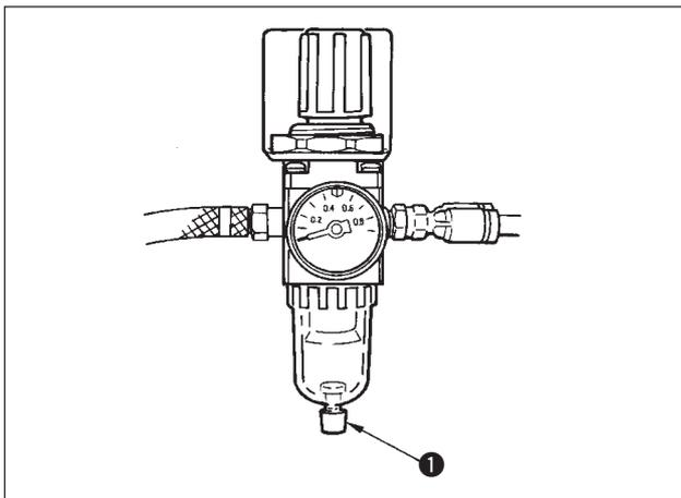
When the regulator becomes filled with water, turn knob **1** for drain counterclockwise.
