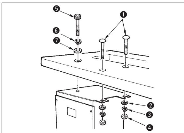
Install the electrical box on the underside of the table at the location illustrated using round-head bolt **1**, plain washer **2**, spring washer **3** and nut **4** supplied with the machine, and using bolt having hexagonal indentation on the head **5**, plain washer **6** and spring washer **7** supplied with the machine.
