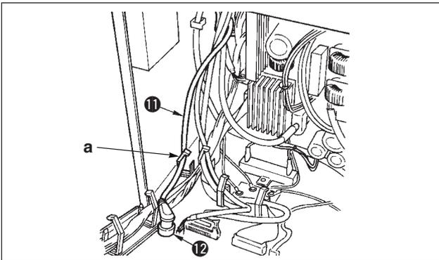
10) Insert gray round connector 7P cord ⑪ coming from the machine head inside the electrical box through front cover through hole B, pass it through cord clamp "a", and insert it into connector CN30 ⑫.
