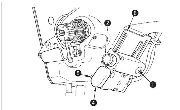
\* The position of reverse feed switch ④ and mirror switch ② can be reversed.
