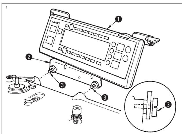
1) Install operation panel **1** on the machine head using screws **3** which have been assembled to panel installing bracket **2**.
