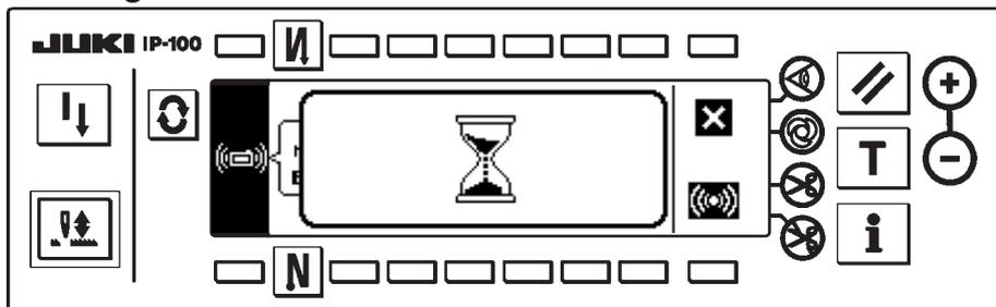
When the screen returns to the communication setting screen after display of the during communication screen, communication is completed.
