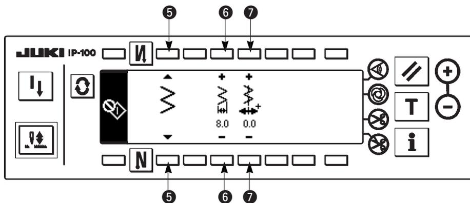
5) Turn ON/OFF the power to return from the hook adjusting mode to the normal sewing mode.
