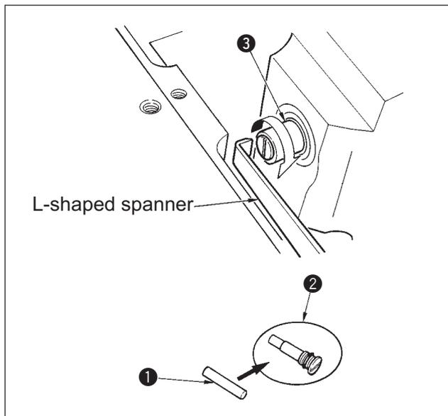
1) Hook shaft oil wick ① is mounted on the top end of hook shaft ③. Remove the needle and the parts around the needle (presser foot, needle, throat plate, feed plate, hook and woodruff plate), put a spanner, top end of which is L-shaped to the groove section of hook shaft oil wick screw ②, turn the handwheel in the normal direction of rotation by hand, and draw out the screw.
