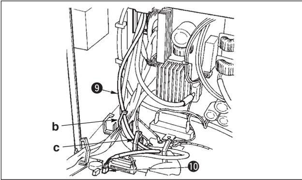
9) Insert black connector 4P white cord ⑨ coming from the machine head inside the electrical box through front cover through hole B, and insert it into connector CN31 ⑩.
