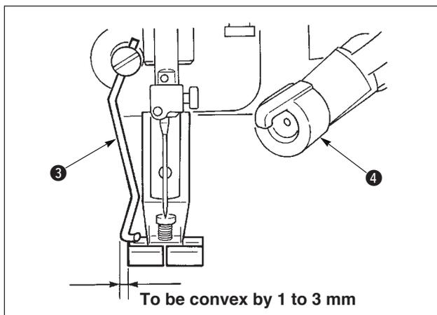
3) Adjust the maximum stroke of the wiper to the position of 1 to 3 mm from the left end plane of the presser of standard delivery.
