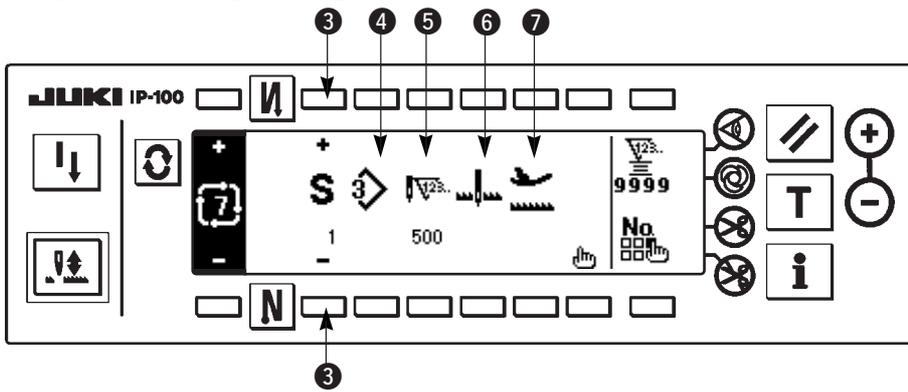
4) Setting of each step can be displayed in the cycle stitching setting screen.
