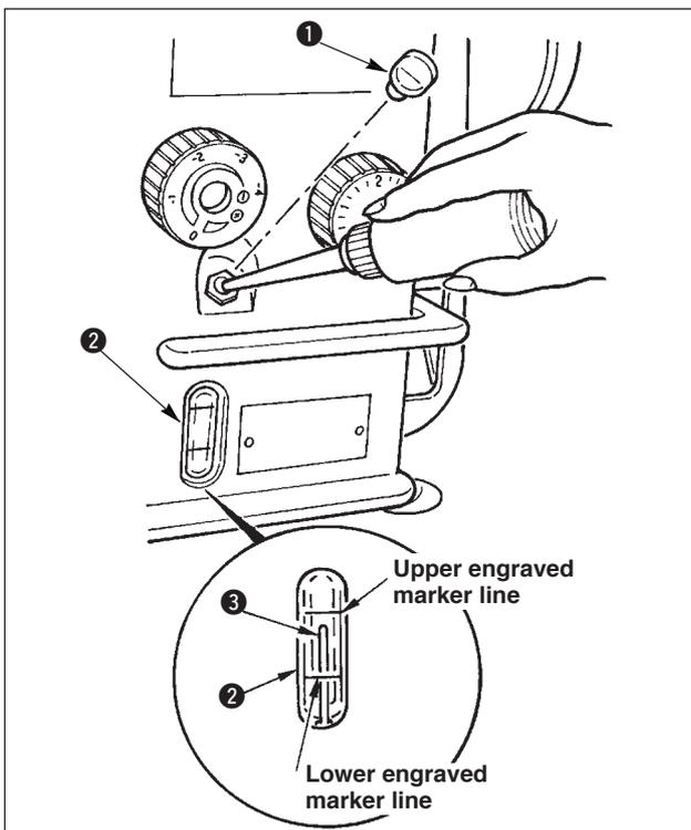
Fill the oil tank with oil for hook lubrication before operating the sewing machine.
