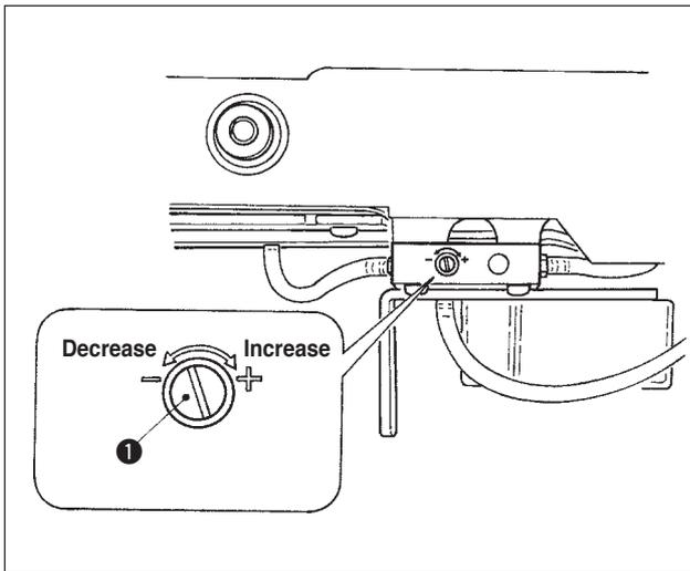
Adjustment of the amount of oil in the hook is performed with oil amount adjustment screw ①.
