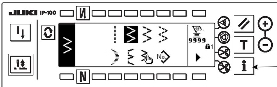
2) Press switch ① for approximately three seconds.
