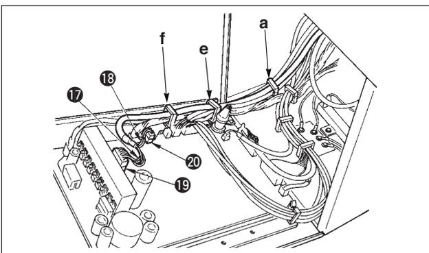
13) Insert white connector 10P cord ⑰ and blue connector 2P cord ⑱ coming from the machine head inside the electrical box through front cover through hole B, pass them through cord clamps "a", "e" and "f", and insert the white 10P into connector CN51 ⑲ and the blue 2P into CN46 ⑳.
