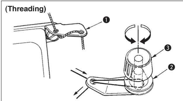
**Note 1.** When winding bobbin thread, start winding in the state that the thread between bobbin and thread tension disk ② is tense.
