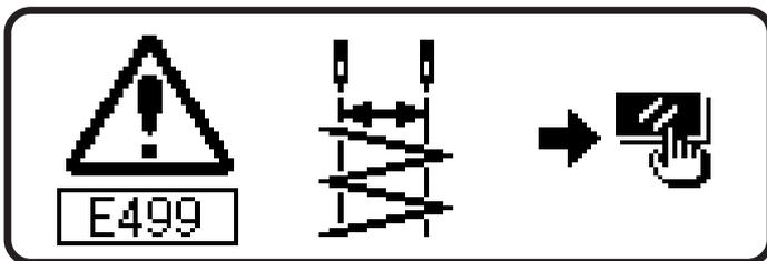
2) Press the reset switch, and remove the cause of error after erasing the error screen.
