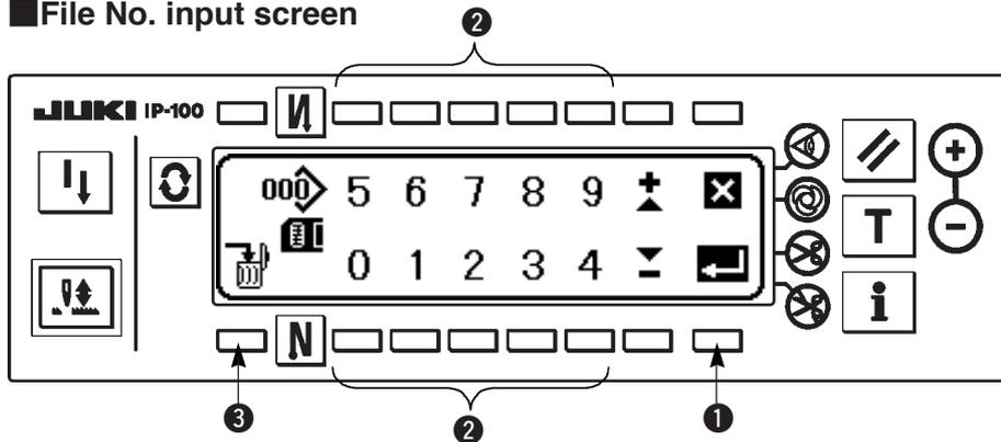
Input the file No. of smart media with ②. The file No. which has been inputted is displayed in . The No. is determined with ① after inputting the file No.
