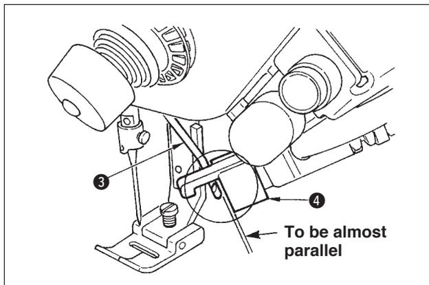
2) The top end plane of wiper ③ should be positioned to be almost parallel to the end plane of clamp head ④. Besides, set the clamp head so that the upper side is the protruding section.
