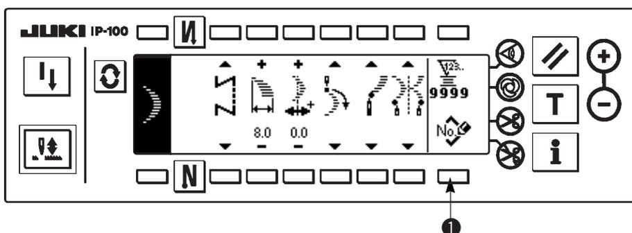
1) Press to display the sewing shape setting screen.
