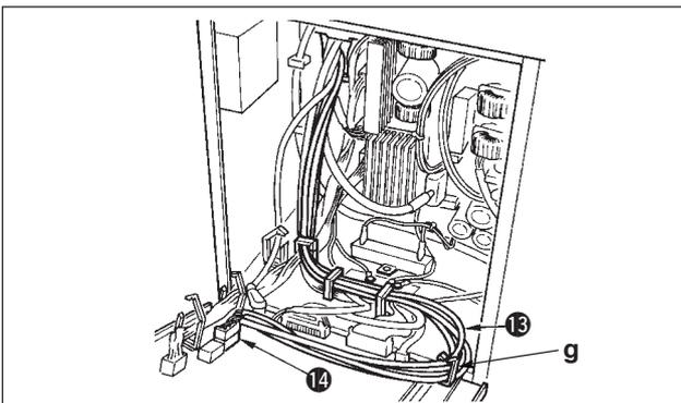
11) Insert white connector 12P cord ⑬ coming from the machine head inside the electrical box through front cover through hole B, pass it through cord clamps "b", "c", "d" and "g", and insert it into connector CN53 ⑭.
