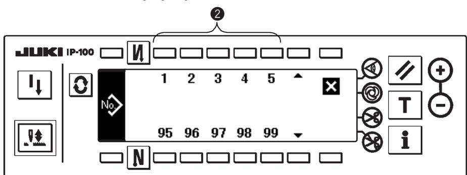
2) Press switch
