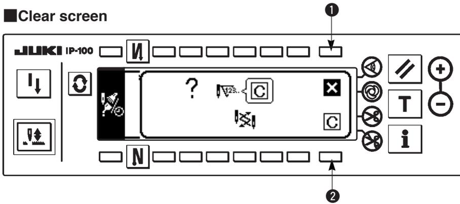
① : The screen returns to the maintenance function screen without performing clearing.
