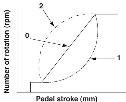
②② **Function added to the needle up / down compensating switch (Function setting No.93 F-MADF)**
