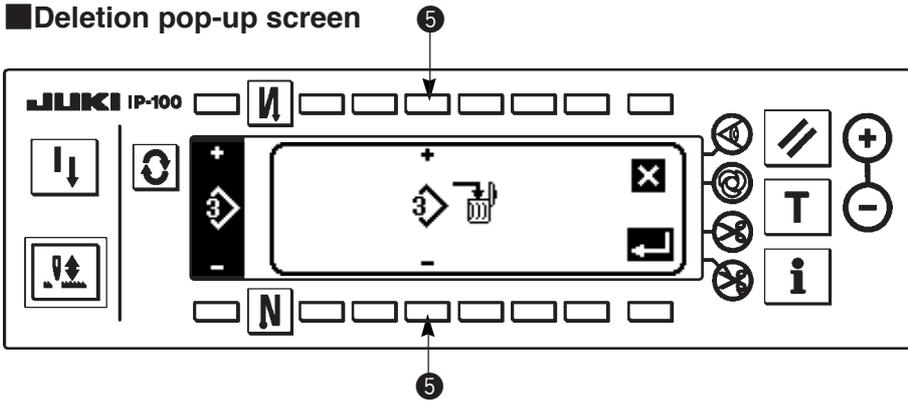
1) Press ② in the copy and deletion pop-up screen to display the deletion pop-up screen.
