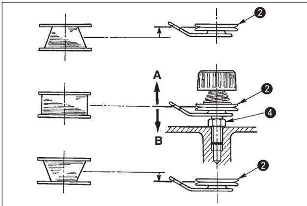
6) In case that the bobbin thread is not wound evenly on the bobbin, loosen the nut ④ and turn the bobbin thread tension to adjust the height of the thread tension disk ②.
