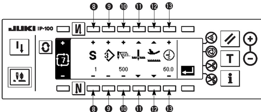
6) Set pattern No., number of stitches, stop position and position of the presser for each step in the cycle stitching edit screen.
