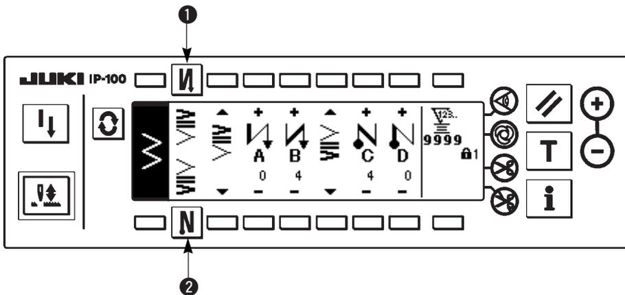
For the reverse feed stitching, there are standard condensation, 2-point condensation and condensation custom.
