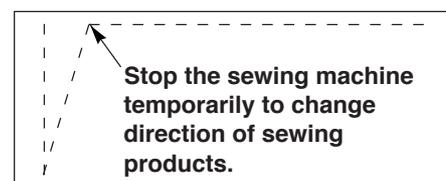
**16 Function of soft-down of presser foot (with AK device only) (Function setting Nos.70 and 49 F-SDFL, T-FLWT)**
