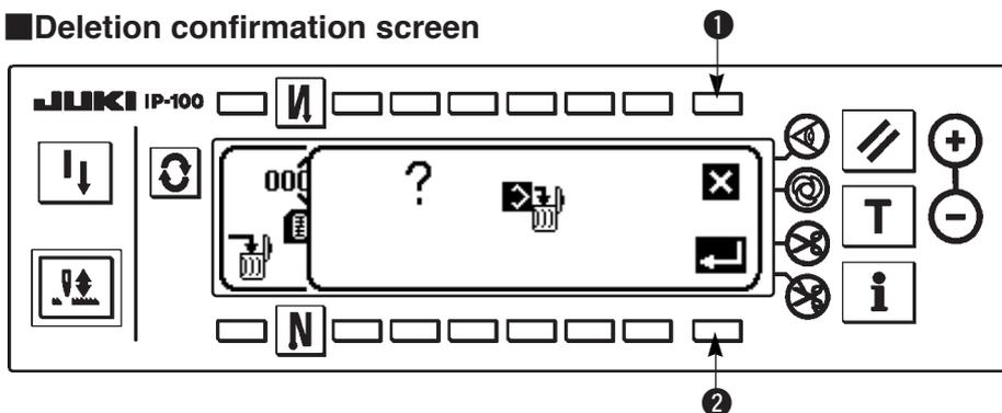
Press ① and the deletion is discontinued. Then the screen returns to the file No. input screen. Press ② and the deletion is executed. Then the screen returns to the file No. input screen.
