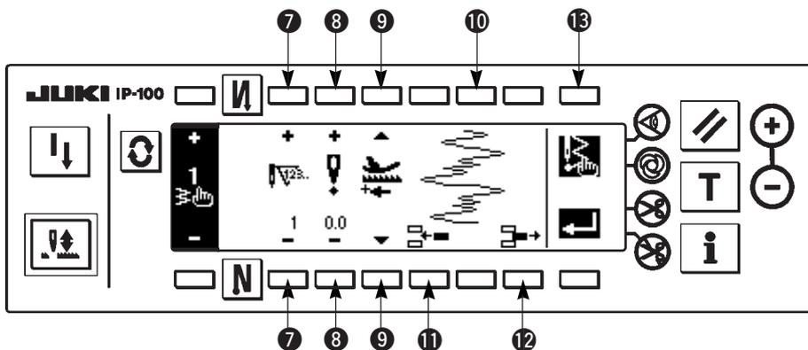
2) Set the needle entry position and sewing direction of each step in the custom pattern edit screen.
