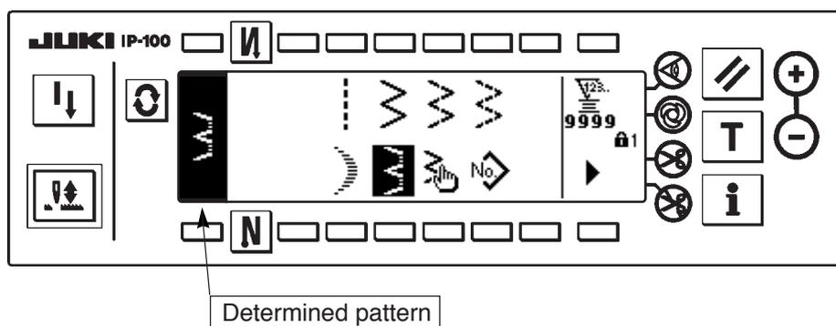
2) As an example, press the left blind stitch key and the screen on the left side appears to determine the pattern.
