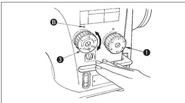
Stitch length can be reduced at the start or end of sewing. This feature is used for fastening stitch.
