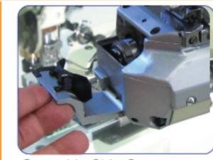
Openable Side Cover Side cover is openable for easy feed dog height adjustment and cleaning.
