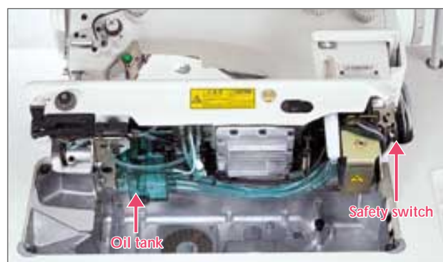
Designed with no oil pan (minute-quantity lubrication type)
