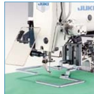
LK-1920SA (Pneumatic separately driven feeding frame)
