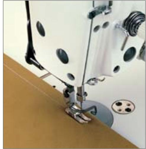
The machine incorporates a newly developed needle-feed mechanism.
